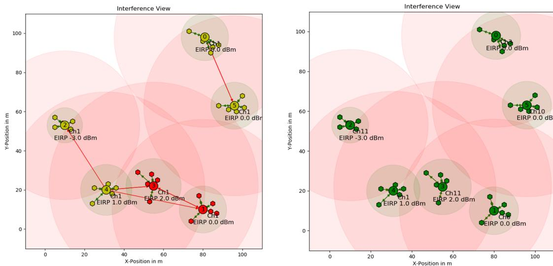
Figure 3: Representation of a typical network graph (left) with initial resource distribution; optimized resource distribution (right). Coexistence states: good (green), medium (yellow), bad (red)
