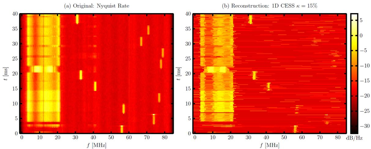
Figure 4 Computed spectrograms of WLAN and Bluetooth signals within the 2.4 GHz bands based on previous sensing: a) sampling with Nyquist rate, b) sampling with 15 % of the Nyquist rate.
